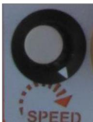
When the machine is in transport position (cage fully lowered), it is possible to regulate the transmission speed by acting on the regulator.
