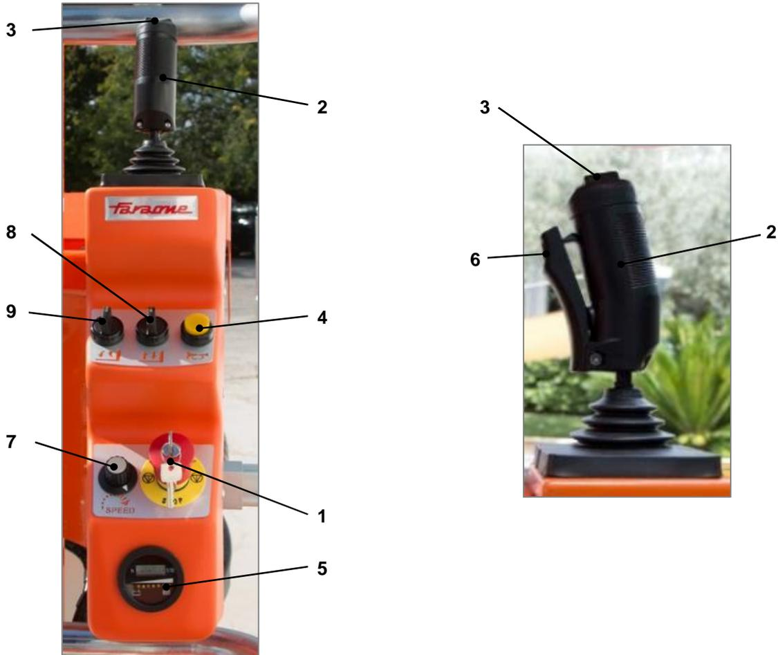
1. Emergency stop button with switch with removable key;
