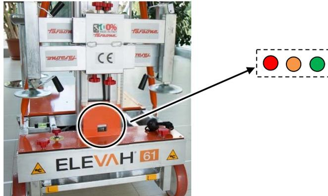
The **RED LED**, when charging the battery, indicates the beginning of the charging cycle. Charging stops automatically with no need for operator action, and is indicated by a **GREEN LED** on.
