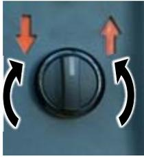
TURN the switch to the LEFT to make the cage DESCEND
