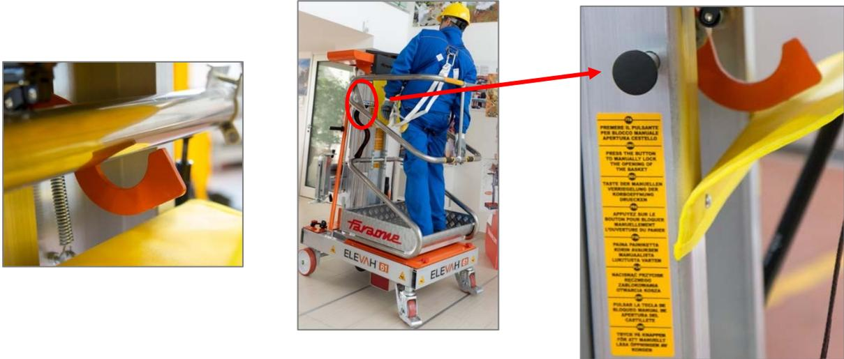
After having pressed the pin, always check that the hook is in the locked position. Following the manual locking of the parapet, the operator will have to manually lower the locking hook until the opening is complete in order to descend from the basket.
