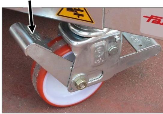
**NOTE:** To release the brakes, push the lever marked “FREE” with your foot (situated on the opposite side of the wheel), bringing the limit switch to its lowest position.
