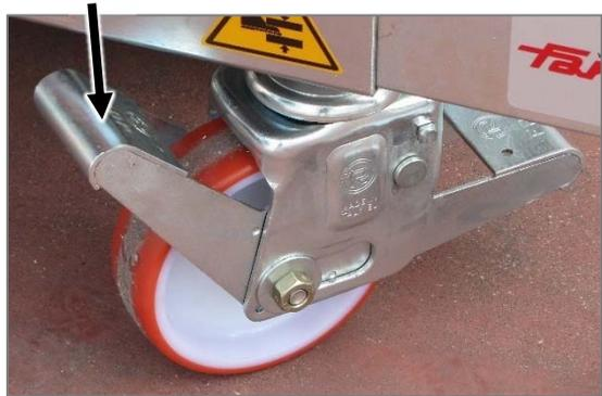
**NOTE:** To release the brakes, push the lever marked “FREE” with your foot (situated on the opposite side of the wheel), bringing the limit switch to its lowest position.
