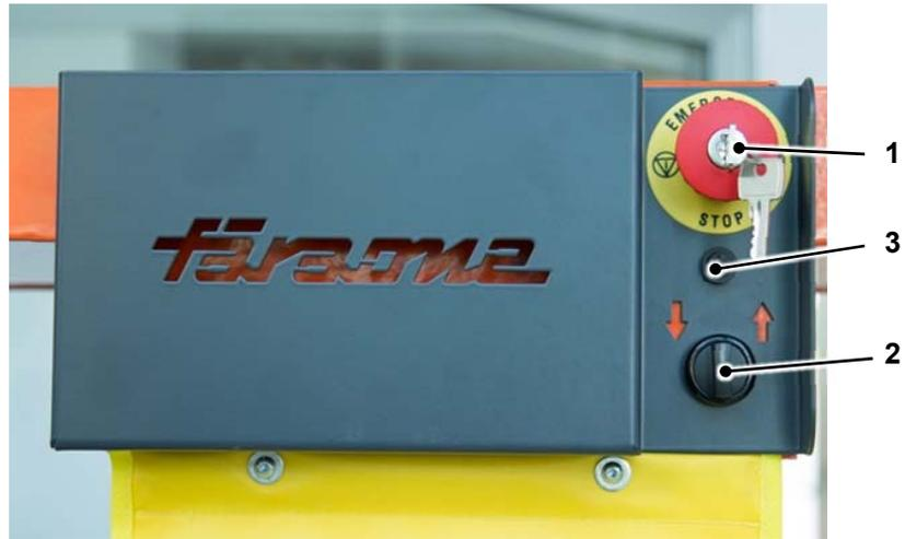
1. Emergency stop/switch-off button with removable safety key
