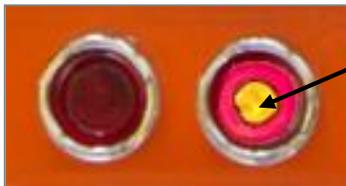
Cage lifting mode enabling LED
