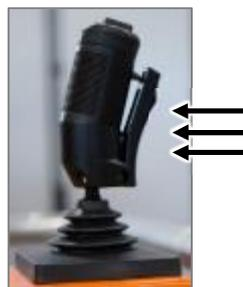
PRESS THE DEAD MAN BUTTON ON THE JOYSTICK, then move the joystick in the required direction. The transmission power is applied proportionally to the shift of the joystick from the centre.
