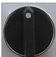
TURN the switch to the RIGHT to make the work platform DESCEND.
