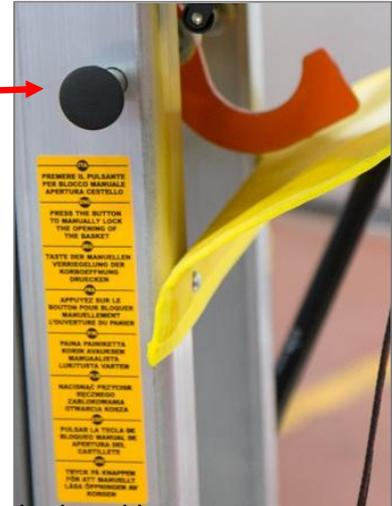
After having pressed the pin, always check that the hook is in its locked position.
