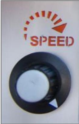
When the machine is in transport position (cage fully lowered) it is possible to regulate the transmission speed from the regulator.
