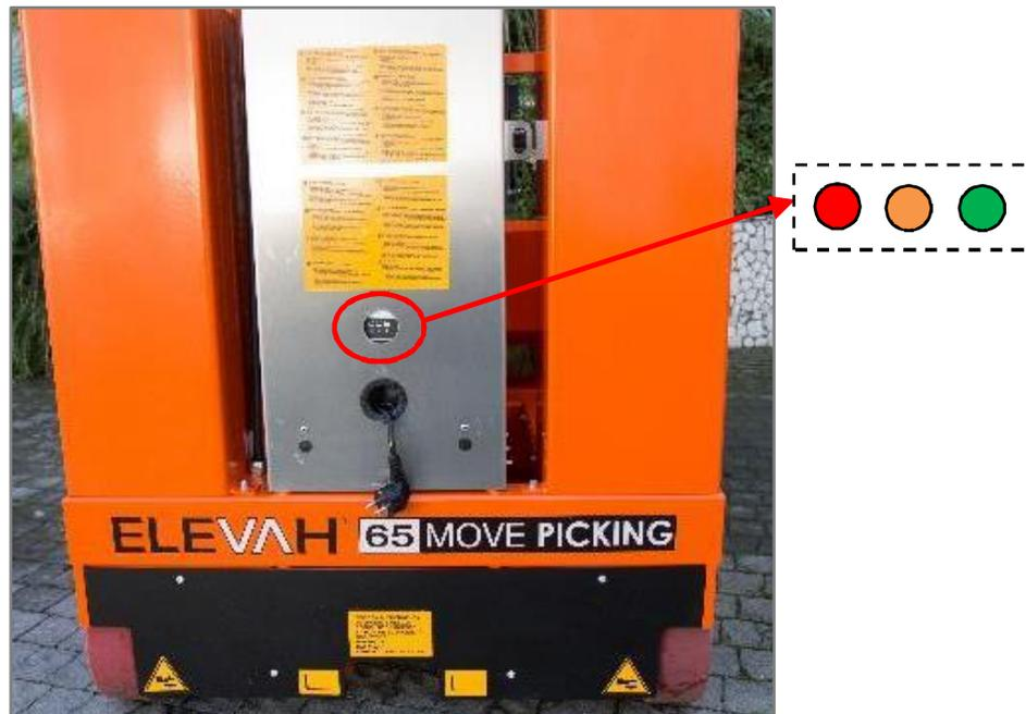
The **RED LED**, when charging the battery, indicates the beginning of the charging cycle.
