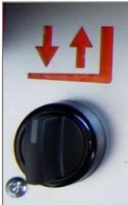
1. Turn the selector to the LEFT to LOWER the loading platform.
