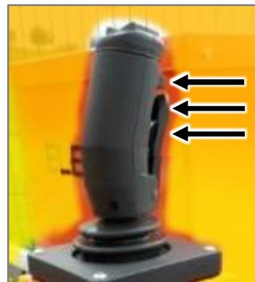
PRESS THE DEAD MAN BUTTON ON THE JOYSTICK, then move the joystick in the required direction. The transmission power is applied proportionally to how far the joystick is shifted from the centre.
