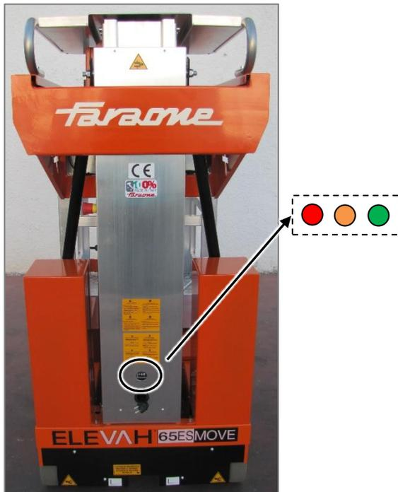
The **RED LED**, when charging the battery, indicates the beginning of the charging cycle.
