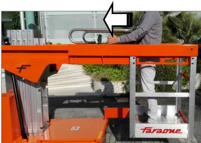
To retract the basket go into the position indicated by the image, hold both handles and:
