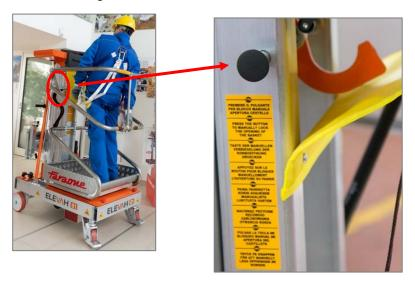
After having pressed the pin, always check that the hook is in the locked position. Following the manual locking of the parapet, the operator will have to manually lower the locking hook until the opening is complete in order to descend from the basket.
