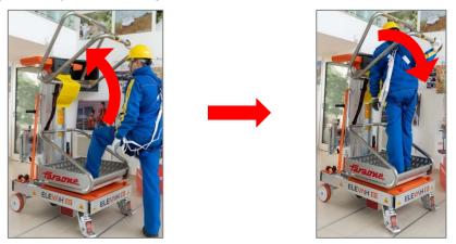
Once the operator climbs on to the cage, the railing is automatically lowered (due to gravity) to the closed position.
