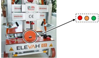
The **RED LED**, when charging the battery, indicates the beginning of the charging cycle. Charging stops automatically with no need for operator action, and is indicated by a **GREEN LED** on.
