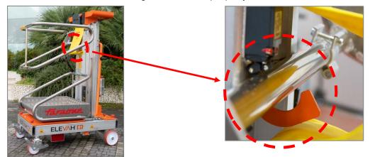
The hook opens automatically when the cage is in the stand-by position (cage on the ground) in order to facilitate climbing up and down (the operator does not need to release the lock by hand) To access the cage, simply lift the railing.
