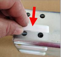
3. Insert the four new pads into the holes (2) made internally, on each side, at the base of the second extension and insert it all the way into the first extension;
