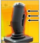
PRESS THE DEAD MAN BUTTON ON THE JOYSTICK, then move the joystick in the required direction.
