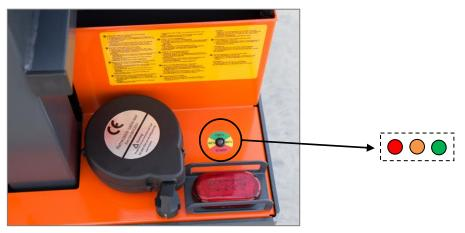
While recharging the battery, the **RED LED** indicates the beginning of the charging cycle. Charging stops automatically with no need for operator action, and is indicated by the **GREEN LED** on.
